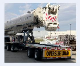
For dollies that are either wide spread or have a rolling tower, if there is a hook block hanging from the boom head it can not be tethered to the dolly. If it's unable to be tethered elsewhere independent of the dolly then the block should be removed
